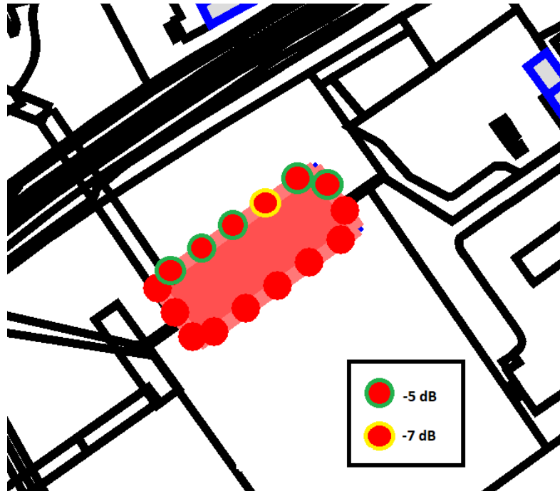
Figure 1.1 Mitigated HVAC Ventilation Units
