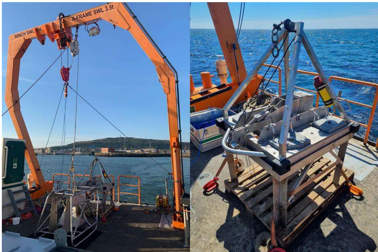
Plate 3 DDC and Hamon Grab mobilised on aft deck of the 'Geo Focus'.
