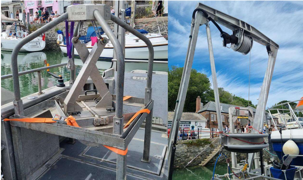
Plate 2 Left: 0.2 m 2 DVV Grab. Right: Equipment dampener mobilised on A-Frame.
