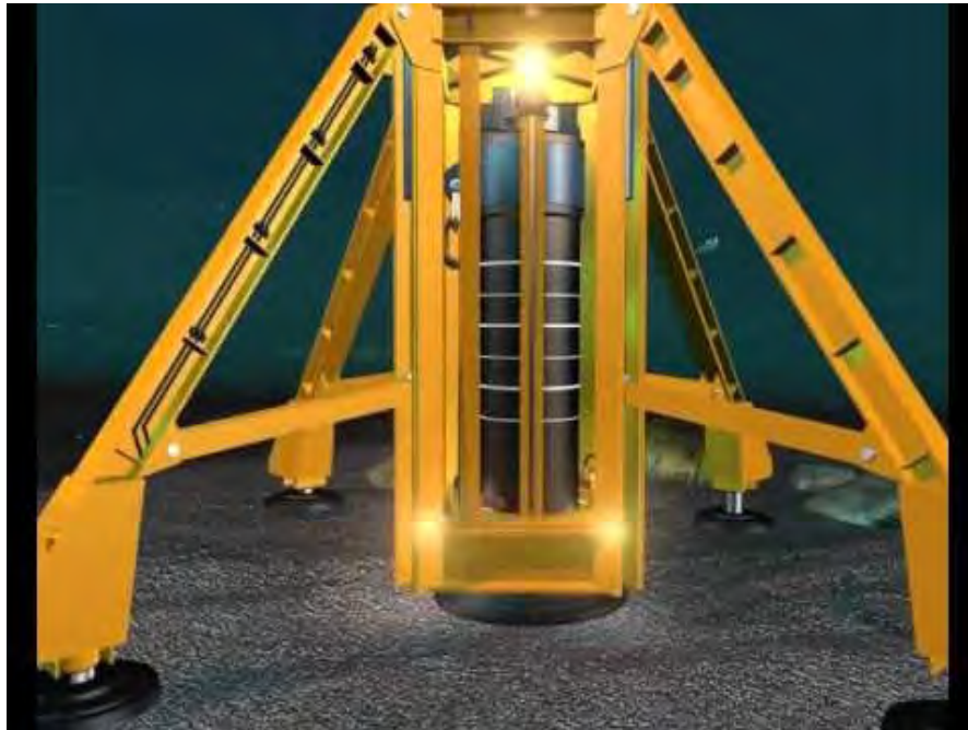
Plate 3.10 Drilled Pile Anchor Example (ABC Moorings, 2022)
