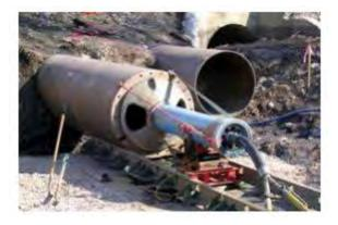
Plate 5.4 Typical pipe ram pneumatic hammer
