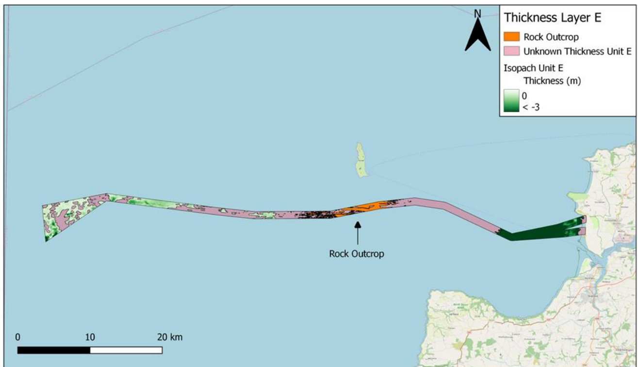
Figure 5-59: Unit E isopach along the ECR (thickness in meters – reflectors R1 and R2 combined)
