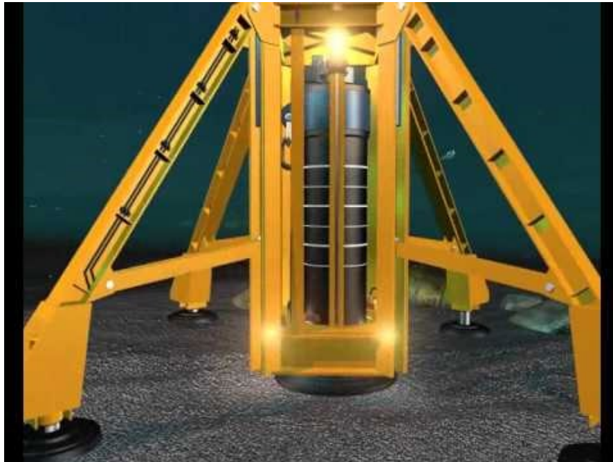
Plate 3.10 Drilled Pile Anchor Example (ABC Moorings, 2022)
