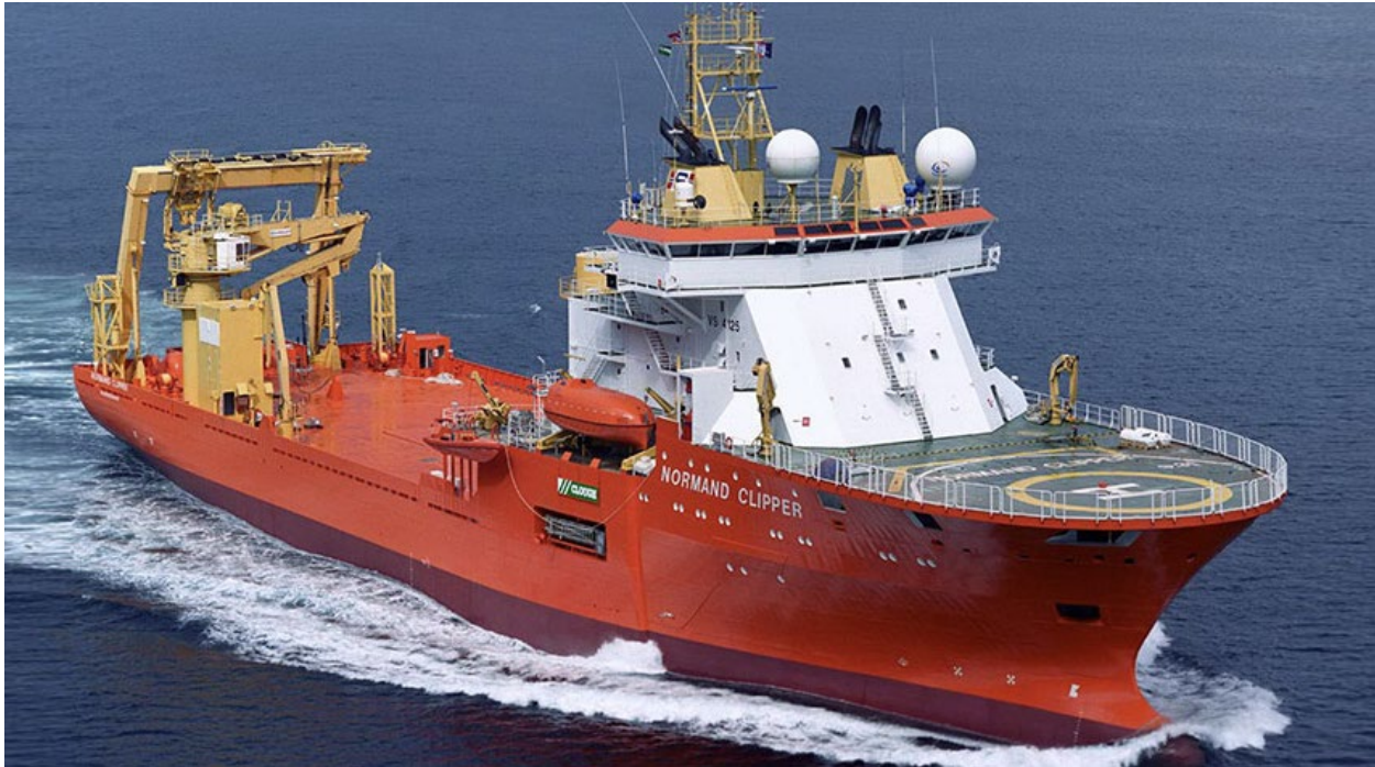
Plate 5.16 A Normand Clipper Cable Lay vessel involved in inter-array cable installation at the Kincardine windfarm
