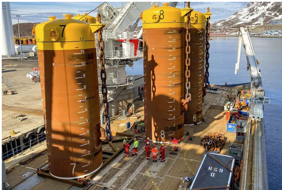
Plate 5.8 Suction Anchor Example (Source: Offshore-Engineer, 2020)
